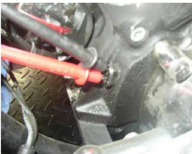
It should be around 16- 20 VAC. Increase RPM and you should see a gain of about 10-20 VAC per 1000 RPM. If not, there could be an issue with the rotor. Although not as common, rotors do have the occasional failure. Magnets can come apart, splines can strip. Take a peek and rule it out.
