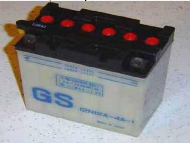
Acid is used in the initial activation, but don't add acid when levels become low. Use distilled water only. Two disadvantages to this type of battery are a susceptibility to static discharge, and if they overheat, can leak acid and make a real mess of things. It's a very effective paint remover!
