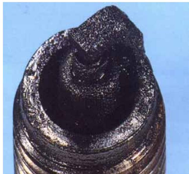
Using plug condition (plug reads) to tune fuel delivery is fairly straight forward. Although not difficult to do with a carbureted bike, it's nearly impossible to accomplish with a fuel injected set up unless the fuel tuner has a manual adjustment for the basic operating ranges. Precise tuning by adjusting maps would be far too tedious and should be accomplished on a dyno, auto-tune systems notwithstanding! We'll cover EFI tuning in a future issue.
