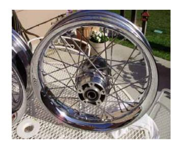
In addition to spokes, faulty wheel bearings can give you trouble. In addition to the requisite service interval, a great time to check both of these is during a tire change. You have the wheel off the bike and access is convenient. The 2000 and later sealed bearing can be inspected by feel. Roll them and they should feel smooth. Worn sealed bearings will have a rough, bumpy feel. 1999 and earlier roller bearings will have to be removed, cleaned, and inspected.
