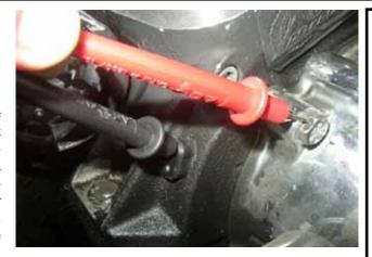
It should read open or zero continuity. If not, the stator is grounded. Now place both probes on the stator pins. It should read close to zero ohms. If the resistance is off the charts (like in the millions of ohms or open) the stator has a break in the coil. If these check out ok, then set the meter to **AC voltage** and with the bike running, measure the voltage output of your stator by placing the probes on both pins/ sockets (see photo 3).
