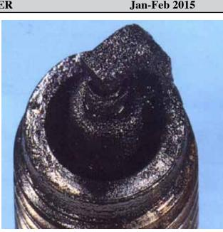
Using plug condition (plug reads) to tune fuel delivery is fairly straight forward. Although not difficult to do with a carbureted bike, it's nearly impossible to accomplish with a fuel injected set up unless the fuel tuner has a manual adjustment for the basic operating ranges. Precise tuning by adjusting maps would be far too tedious and should be accomplished on a dyno, auto-tune systems not withstanding! We'll cover EFI tuning in a future issue.
