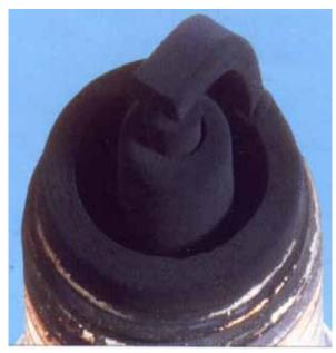
Plugs that are covered in a wet black deposit are oil fouled. This is a result of worn piston rings, valve guides,
