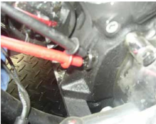
It should be around 16- 20 VAC. Increase RPM and you should see a gain of about 10-20 VAC per 1000 RPM. If not, there could be an issue with the rotor. Although not as common, rotors do have the occasional failure. Magnets can come apart, splines can strip. Take a peek and rule it out.
